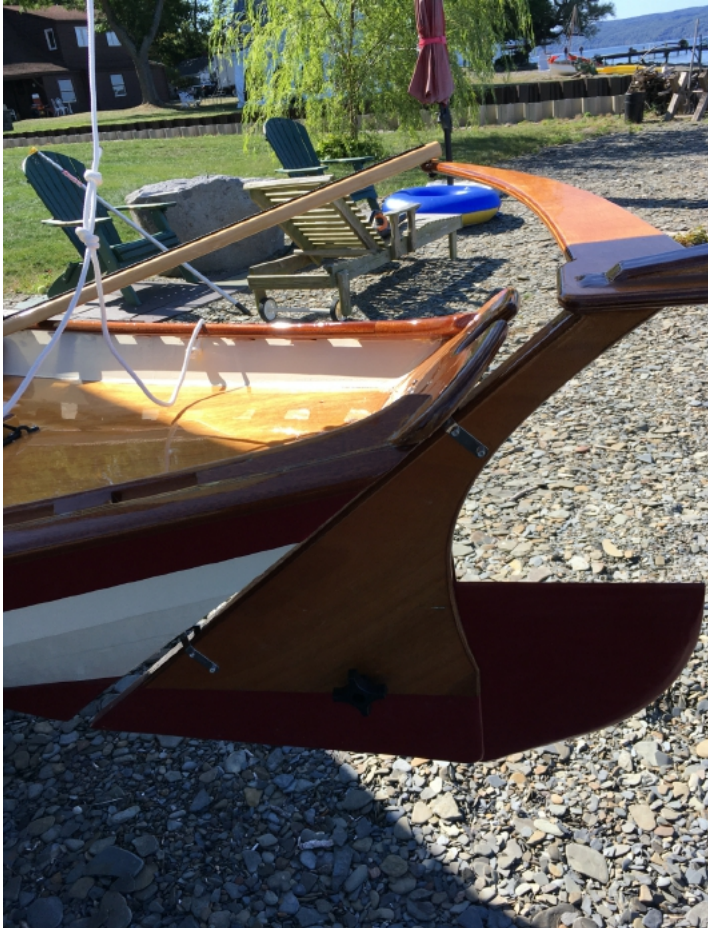
Photo 10: The dory features a yoke and draglink tiller and pop-up rudder.
