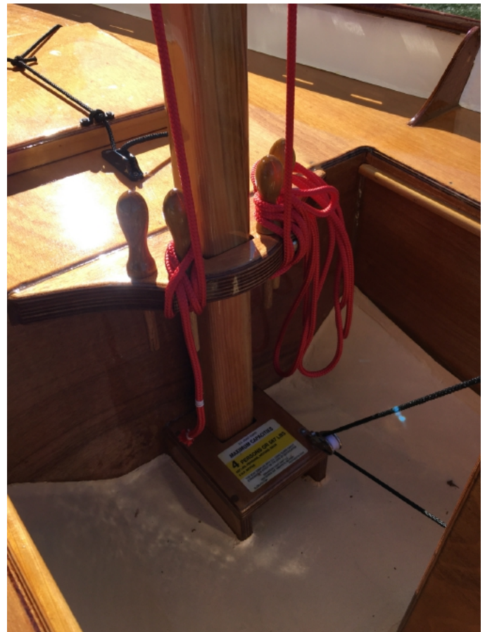
Photo 9: Traditional belaying pins are an efficient way to manage halyards and downhauls.
